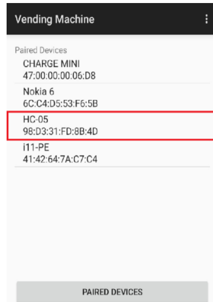
Figure 7. HC-05 Bluetooth Pairing with Vending Machine
